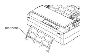
2. Hold down the LF/FF button to eject the remaining labels from the printer.
